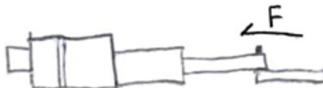
Figure 8: Linear Actuator Driving a Guide Rail
