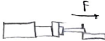
Figure 9: Pneumatic Actuator Driving a Guide Rail
